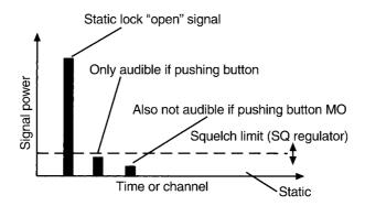
Advice; the SQ regulator only functions in the described ways if the received evaluation of the CTCSS and DCS pilot procedure is switched off (indicator TSQ cannot be seen on the display). If it is switched on, the loudspeaker on the equipment reacts when receiving the suitable pilots only! The MO button also works with activated pilots and offers the opportunity to listen into the channels.
